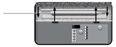
3. Connect the wires of the thermostat to the two screw terminals next to the power adapter plug. (see figure below).
